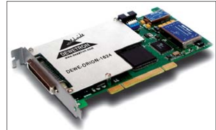
Figure 3. DEWE-Orion-1624 A/D converter
